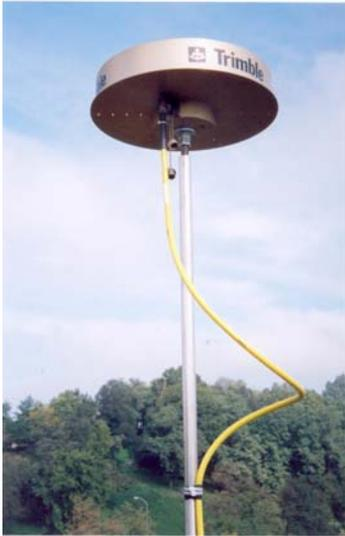
New University of Pittsburgh Seismic Station Second Picture: New CORS (continually operating recording station) GPS base station being run in cooperation between the National Geodetic Survey, PennDOT and G&PS.
