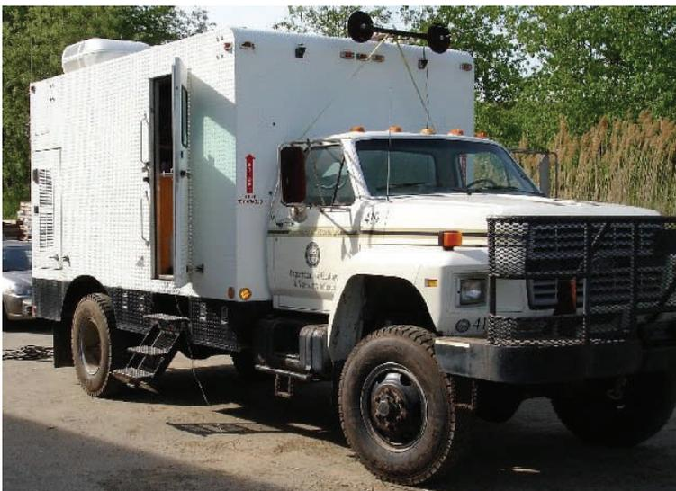
*The WesternGECO-donated F700 seismic recording truck allows recording of up to 3000 channels of 24-bit digital data simultaneously. It has a 24 kV or can be run via shore power.*
