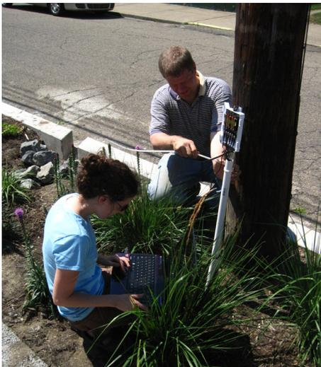
Krissy Hopkins and Dan Bain install soil moisture sensors to monitor a bioswale in Greenfield, PA. July 2012
